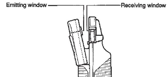
Figure 4: Illuminating/measuring system of the SPAD-502Plus
