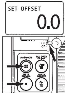
2. Set the compensation value using **ALL DATA CLEAR** and **DATA DELETE**. The compensation value will increase by 0.1 each time **ALL DATA CLEAR** is pressed; value will decrease by 0.1 each time **DATA DELETE** is pressed. The compensation value can be set between -9.9 and 9.9 in 0.1 steps. The compensation value is set to 0.0 at the factory.
