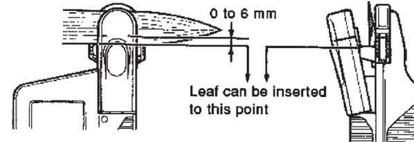
When not using the depth stop, remove it, turn it around (with the tabs facing away from sample slot) and replace it on the measuring head.
