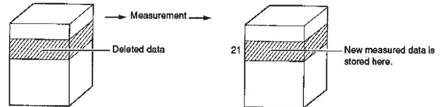
2. If the display is changed to another data number by using the DATA RECALL, the remaining data in memory will be shifted up to fill the space for the data number from which data was deleted and the new measured data will be stored in the space for the next empty data number.
