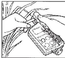
3. Press on the finger rest to close the measuring head. Hold it closed until a beep sounds and the measured value appears in the display. The measurement will automatically be stored in memory.
