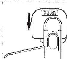
2. Perform calibration. With no sample in the sample slot, press on the finger rest to close the measuring head and hold it closed until a beep sounds and the display shown at right appears.
